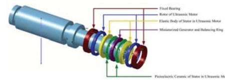
Fig. 1. Schematic illustration of a self-powered balancing ring in a rotor system.
