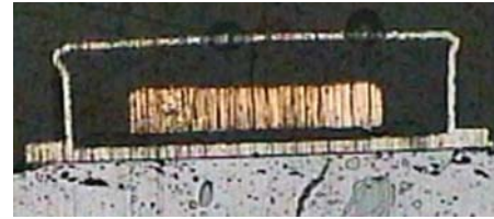
Figure 1: Cross-section of fabricated single turn inductor.
