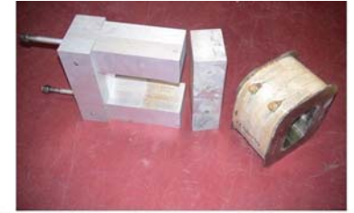
Figure 2. Picture of the disassembled transformer: coil and U and I parts manufactured with laminated silicon steel plates.
