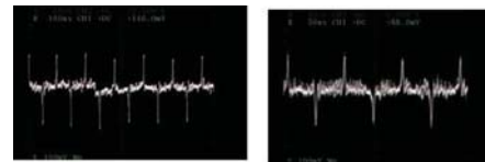
Figure 1. Unstable waveform after 339hours of drive operation.
