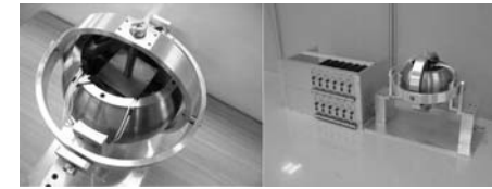
The spherical motor structure and the current driver
