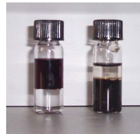
Figure 2: Left: top: FePt@Au dispersed in hexane, bottom: water. Right: top: hexane, bottom: FePt@Au dispersed in water.
