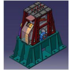
Fig. 3 3-D drawing of the SLSM test wheel construction.
