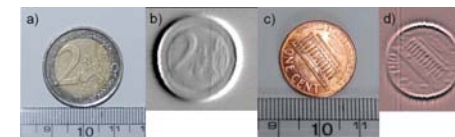
Fig. 3 Optical photo images a), c) and scanned images b), d) by inductive thin film sensor, respectively.
