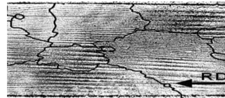
Fig. 1. Static domain structure aligned with rolling direction (RD) showing grain orientation in 40 mm x 30 mm GO sample (grade M4)
