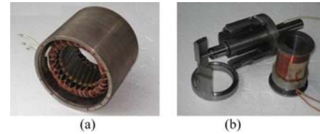
Fig.3 1-kW prototype assembly. (a) Stator. (b) Rotor.
